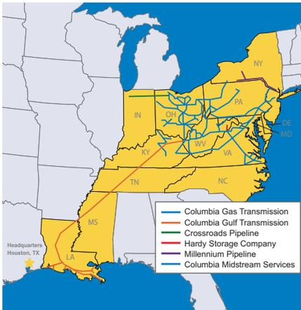
Columbia Gulf Transmission operates approximately 2,400 miles of high pressure natural gas transmission pipelines and 10 compressor stations with nearly half a million horsepower in Louisiana, Mississippi, Tennessee, and Kentucky. The company provides natural gas transportation service to local gas distribution companies and large volume customers to help meet U.S. energy needs.
