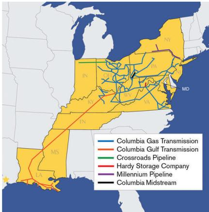
Columbia Gulf Transmission operates approximately 2,400 miles of high pressure natural gas transmission pipelines and 10 compressor stations with nearly half a million horsepower in Louisiana, Mississippi, Tennessee, and Kentucky. The company provides natural gas transportation service to local gas distribution companies and large volume customers to help meet U.S. energy needs.
