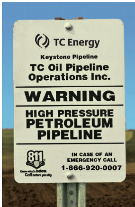
Typical TC Energy Keystone marker sign on the pipeline right of way (ROW) at road / railway and canal crossings
