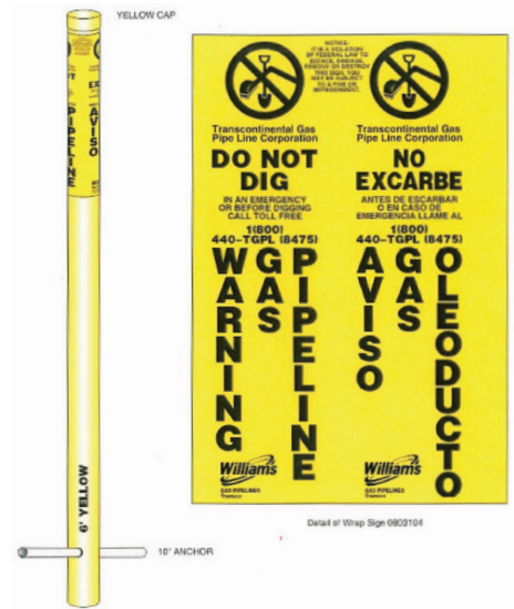
Williams Gas Pipeline - Transco Pipeline Markers
