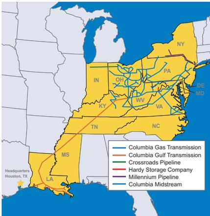
Columbia Gas Transmission transports an average of three billion cubic feet of natural gas per day through a 12,000-mile pipeline network and 103 compressor stations serving hundreds of communities in 10 states. Our customers include local gas distribution companies, energy marketers, electric power generating facilities and hundreds of industrial and commercial end users.
