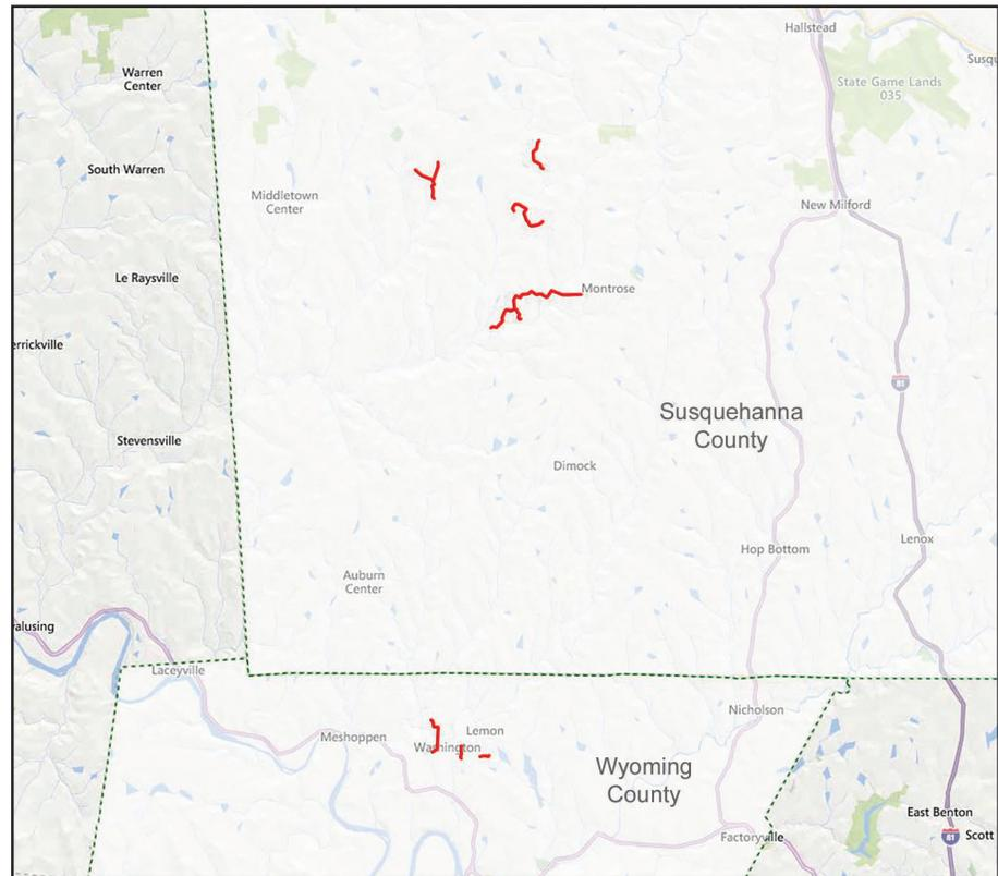
Susquehanna county is comprised of approximately 12 miles of 6", 8" and 10" natural gas gathering pipelines operating at 500#. Wyoming county is comprised of approximately 3 miles of 8" and 10" natural gas gathering pipelines operating at 1200#.
