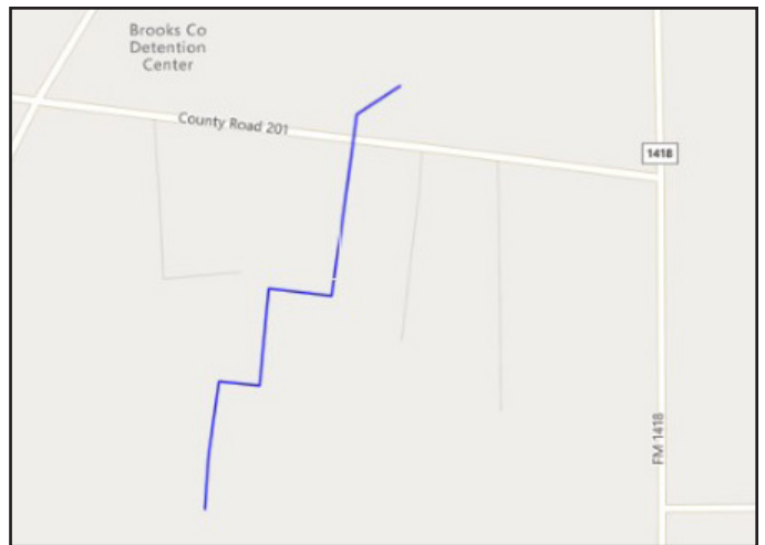
The Church of the Brethren Pipeline System is a Gathering Pipeline that is 4.5” in diameter in Brooks County.
